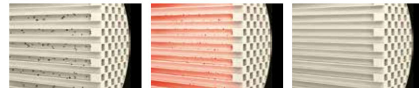
1. Particulate matter trapped 2. Regeneration starts 3. Regeneration completes*
